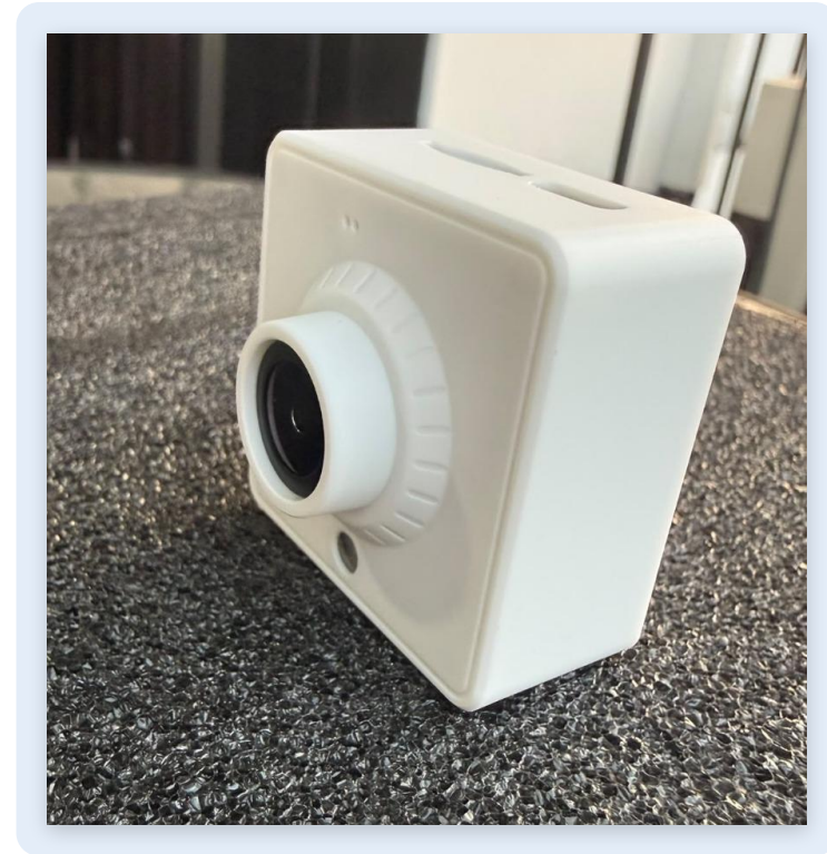
Front shell, lens barrel and status light, as assembled
