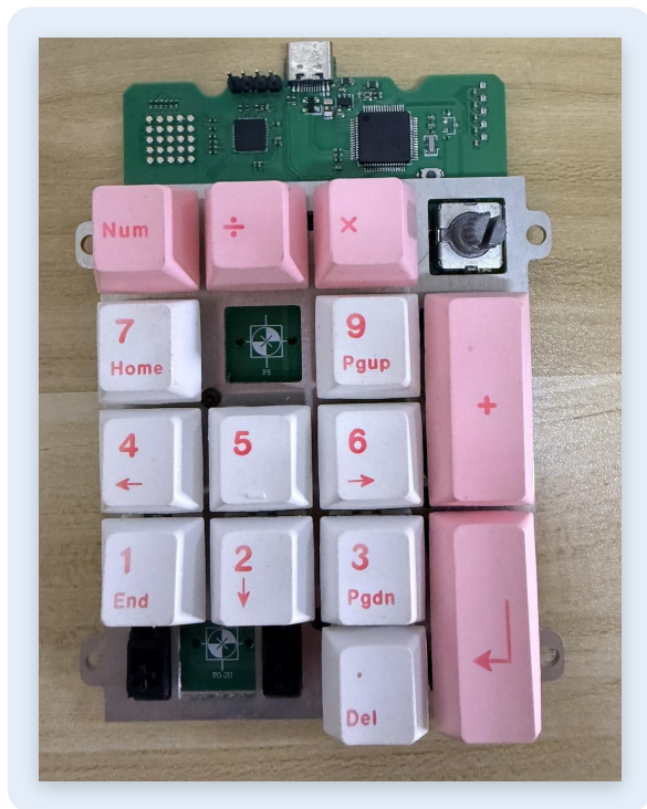
Assembled prototype — board, plate, stabilisers, encoder
