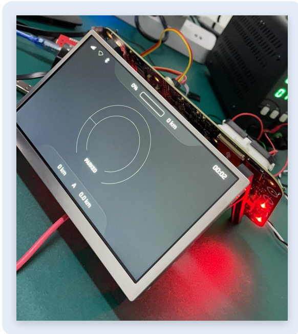
Bring-up rig — panel, carrier board and bench supply
