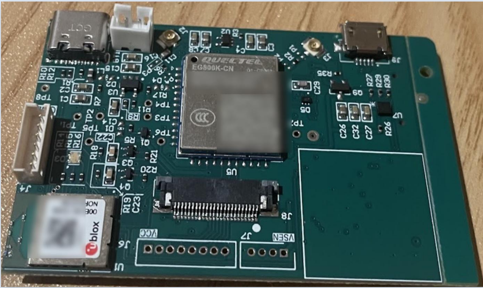
Collar mainboard — cellular, BLE and charge management
